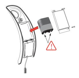
4. Insert a new 6 Volt Type 2CR5 Lithium Battery. The red LED will flash for one (1) minute. Reinstall Battery Cover. Reconnect electrical lead at connector if previously disconnected. Reinstall Throat Plate. If LED doesn't flash or if it just lights up, remove and then reinsert the Battery. If water flows continuously after inserting the new Battery and opening the Supply Stops, remove and then reinsert the Battery.
