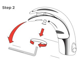
2. Loosen Screw with hex wrench. Remove Throat Plate. Disconnect electrical lead at connector if required.
