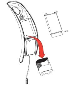
3. Remove Battery Cover using a No. 1 Phillips head screwdriver. Remove old Battery and dispose of properly.
