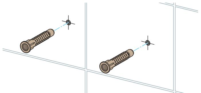
**4b.** Mount the control box on the wall. Drill two 1/8" (3mm) holes as shown, and push drywall anchors into each hole. Secure the control box to the wall with the drywall screws.
