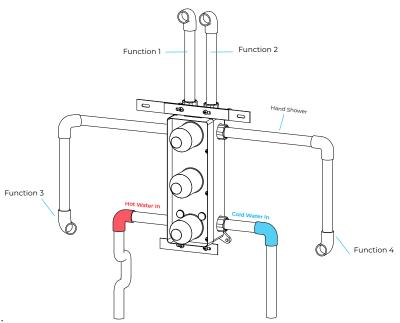
The minimum required water pressure is 0.05 MPa (0.5 bar). Flow rate 2.5 GPM (9.5 LPM).
