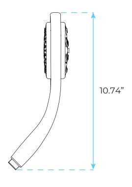
Flow rate 2.0 GPM (9.5 LPM).
