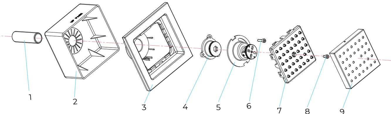
**Parts :** 1.Pipe, 2.Plastic box, 3.Decorative plate, 4.Connector, 5.Body, 6.Bolt #6, 7.Outlet face, 8.Bolt #8, 9.Outlet face
