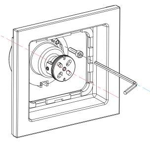
**Step 7:** Screw the bolt #6 into the body. Make sure the body and the connector are tight. The decorative plate should now be secure and will not move
