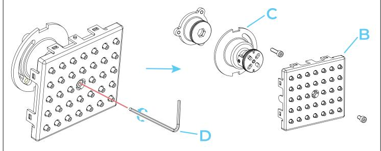
Step 2: Remove the screws from the outlet face (B) and connector body (C) with the Allen key (D).
