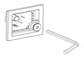
**Step 5:** Screw the connector into the pipe with H10 wrench
