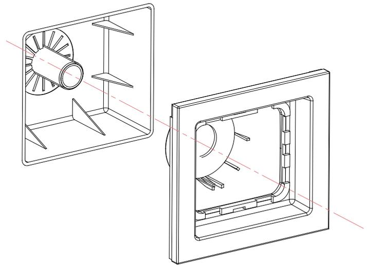
**Step 4:** Install the decorative plate assembly into the plastic box. Make sure the position is correct
