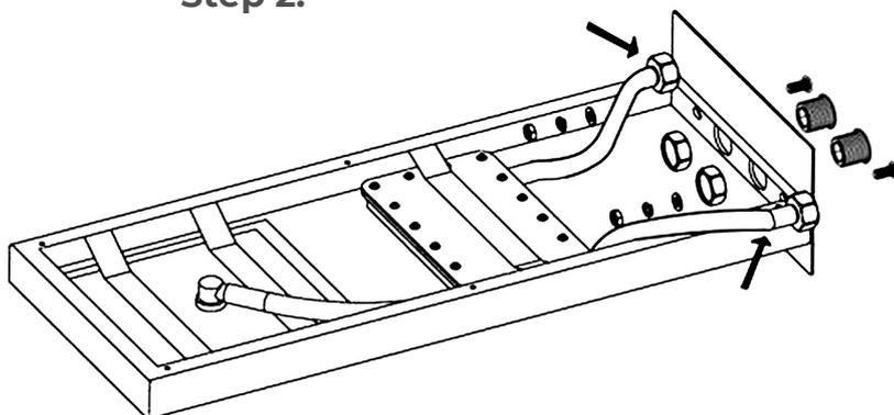
Two inlet fittings are connected to the pipe joint of the wall; then the nut, expansion screw, and inlet pipe are connected.
