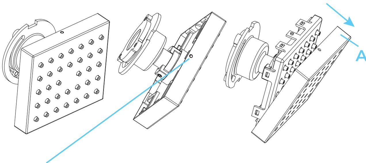
**Step 1:** Push the hole. Remove the decorative plate (A) out of the body
