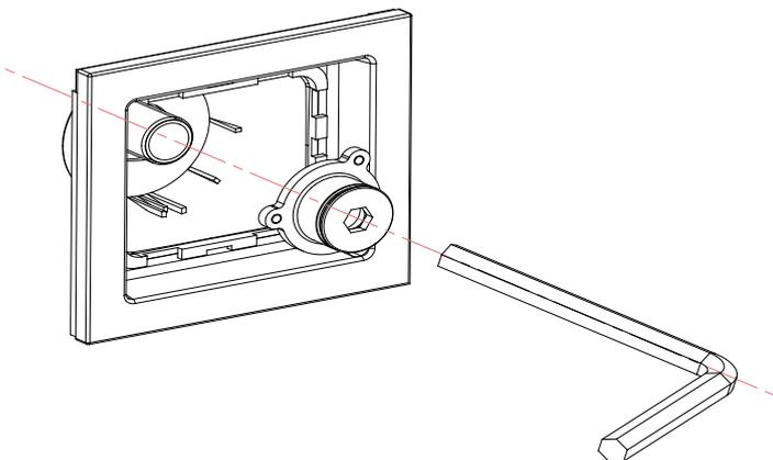
**Step 5:** Screw the connector into the pipe with H10 wrench
