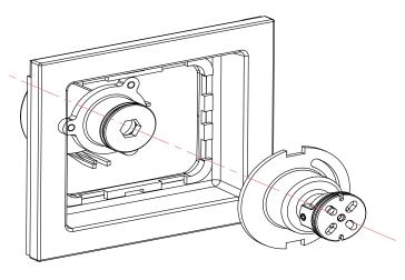
**Step 6:** Install the body assembly to the connector
