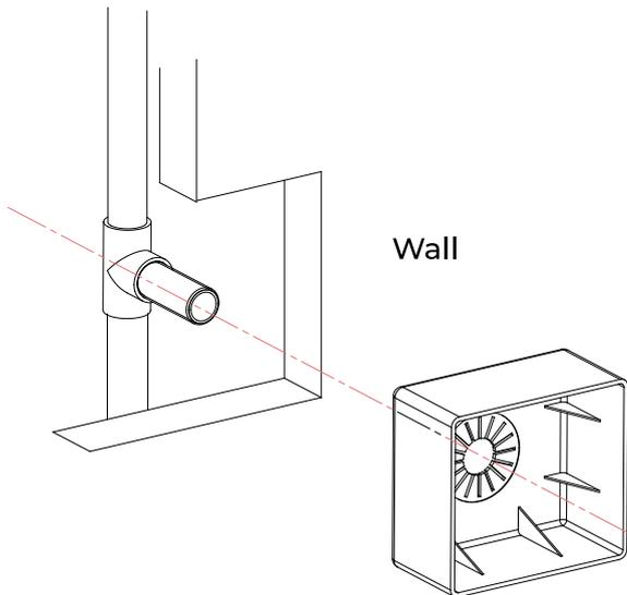
**Step 3:** Push the plastic box into the wall
