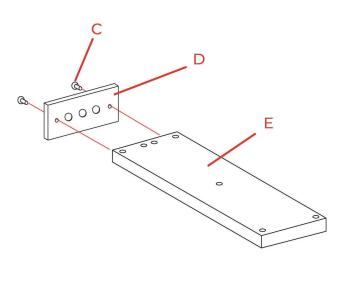
Fix the escutcheon (D) to the showerhead (E) with screws (C).
