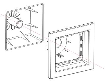
**Step 4:** Install the decorative plate assembly into the plastic box. Make sure the position is correct
