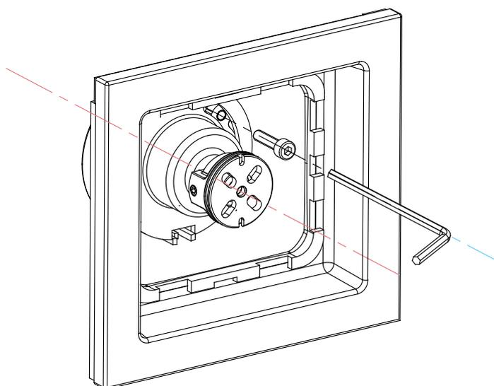
**Step 7:** Screw the bolt #6 into the body. Make sure the body and the connector are tight. The decorative plate should now be secure and will not move
