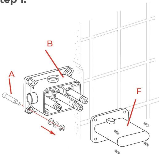
Remove the protective cover (F). Mark the positions and drill holes to suit the anchors (A). Install the anchors (A) and fix the rough-in valve (B) into the wall with screws. Use a level to ensure that the rough-in valve (B) is straight and level. (Important: Flush the water supply to remove any dirt and debris before installing the valve body).
