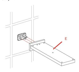
Remove the protective cover when the finished wall is completed. Then, install the showerhead (E) and press it against the finished wall.
