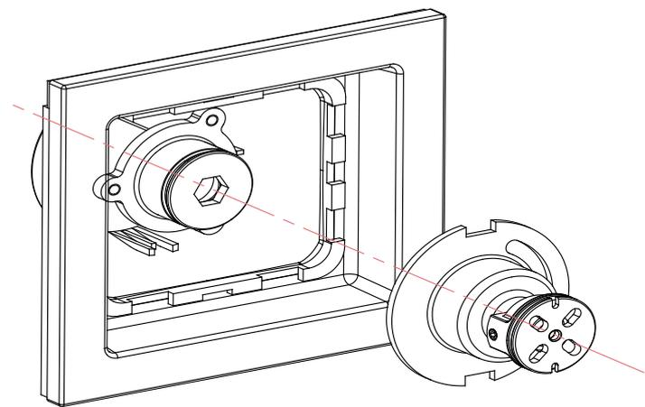
**Step 6:** Install the body assembly to the connector
