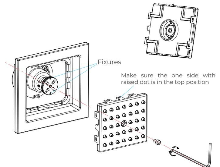
**Step 8:** Install the outlet face assembly to the body. Make sure the outlet face is fully seated onto the body. Screw the bolt #8 through the outlet face into the body (*Do not over tighten*)
