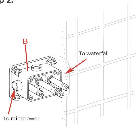
Wrap Teflon tape around the pipe threads and connect water supply lines and in-wall pipes (not included) as desired to the rough-in valve (B). Turn on the water supply and open the cartridge to check for leakage. Then put on the protective cover and finish the wall surrounding the valve. (Note: Test the water pressure after the pipe connections have been made and before the finished wall material is installed).
