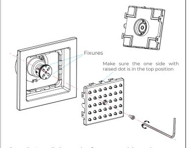
**Step 8:** Install the outlet face assembly to the body. Make sure the outlet face is fully seated onto the body. Screw the bolt #8 through the outlet face into the body *(Do not over tighten)*
