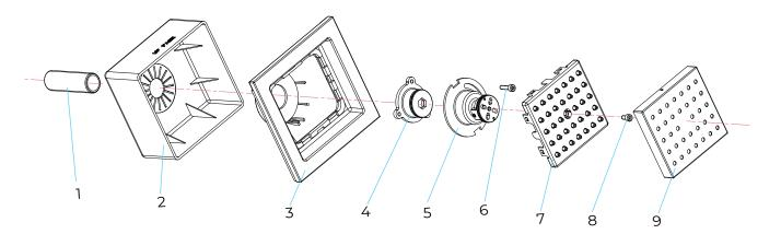
**Parts:** 1.Pipe, 2.Plastic box, 3.Decorative plate, 4.Connector, 5.Body, 6.Bolt #6, 7.Outlet face, 8.Bolt #8 9.Outlet face
