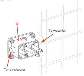
Wrap Teflon tape around the pipe threads and connect water supply lines and in-wall pipes (not included) as desired to the rough-in valve (B). Turn on the water supply and open the cartridge to check for leakage. Then put on the protective cover and finish the wall surrounding the valve. (Note: Test the water pressure after the pipe connections have been made and before the finished wall material is installed).
