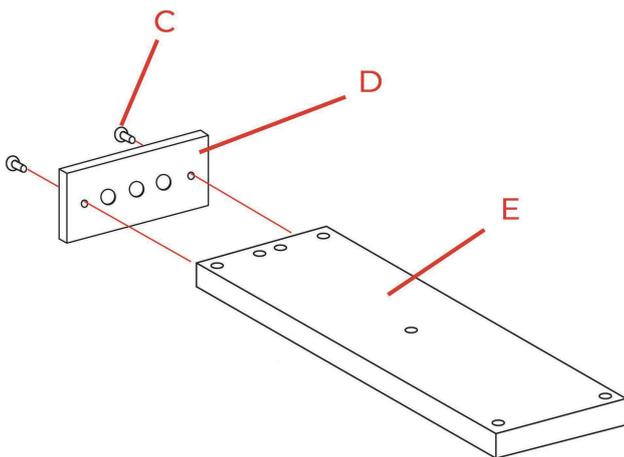
Fix the escutcheon (D) to the showerhead (E) with screws (C).
