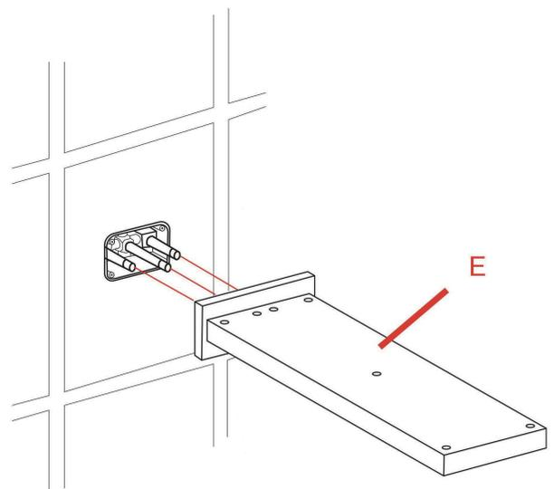
Remove the protective cover when the finished wall is completed. Then, install the showerhead (E) and press it against the finished wall.
