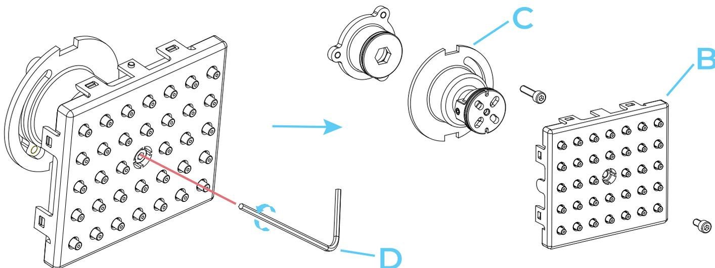
**Step 2:** Remove the screws from the outlet face (B) and connector body (C) with the Allen key (D).
