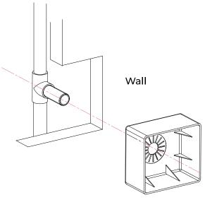
**Step 3:** Push the plastic box into the wall **IMPORTANT:** Please make sure the UP FACE marking is in the top position
