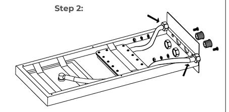
Open the top cover and drill according to the marked position.
