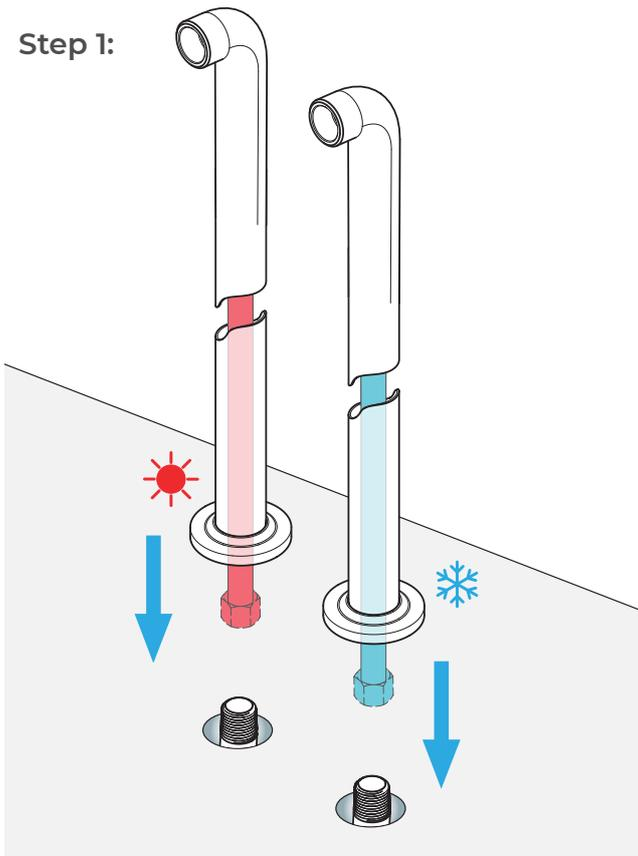
Insert the base cover plate and connect the shower legs to the Hot & Cold water supply lines.
