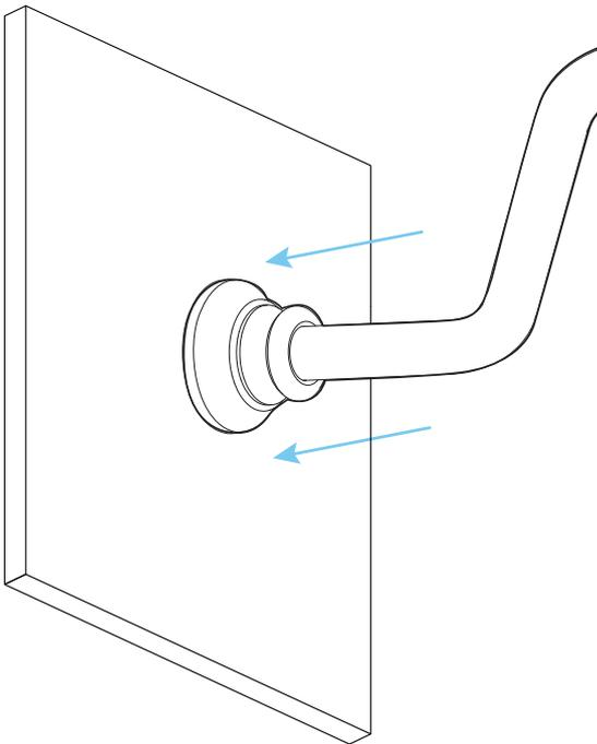
Position the arm vertically and push trim ring into place. Use wrenching flats to tighten.
