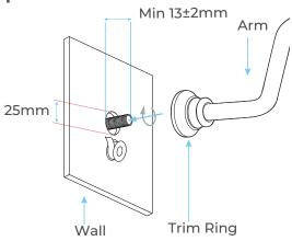
Slide chrome trim ring onto the appropriate end of the arm. Ensure that a minimum of 13±2mm of 1/2" connection thread protrudes past the finished wall. Simply screw the arm onto the connection. Correct water proofing must be applied.
