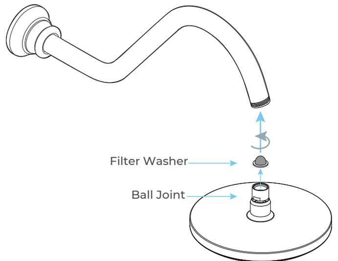
Remove the protective cap from the showerhead ball joint and screw the unit onto the overhead arm ensuring the filter washer is in place.
