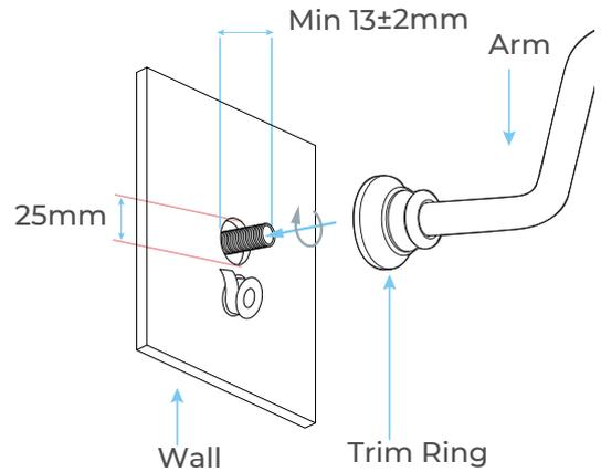
Slide chrome trim ring onto the appropriate end of the arm. Ensure that a minimum of 13±2mm of 1/2" connection thread protrudes past the finished wall. Simply screw the arm onto the connection. Correct water proofing must be applied.
