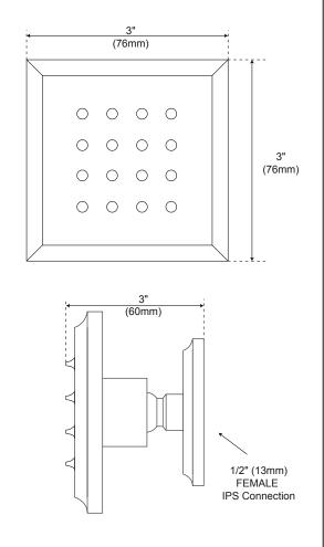
Flow Rate: 2.0 GPM / 7.6 LPM
