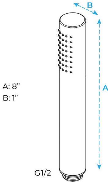
The minimum required water pressure is 0.05 MPa (0.5 bar).
