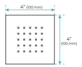
Thread Interface Size: G 1/2 Inch Installation Type: Wall Mounted
