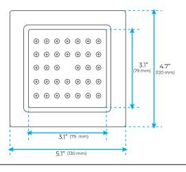
**FEATURES** Material: Brass Base Plate Height: 5-1/8" Base Plate Width: 5-1/8" Jet Surface Area: 3-1/8" Surface Depth: 1/4" Adjustment Angle: 5° Male NPT Connection: 1/2"
