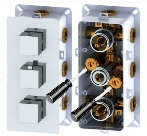
The thermostatic shower mixer is equipped with two stop valves on the inlet side. When you need to repair and maintenance the shower mixer and fittings on each shower mixer, you only need turn the thermostat clockwise two stop valves, you can turn off the water.
