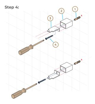
**4.** Insert anchors (1) into drilled holes. Slide covers (2) over brackets (3), and insert screws (4) into bracket/cover assembly. Secure assembly to wall with screws.
