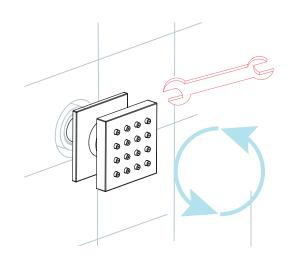
Step 4: Screw the Body spray tightly into the female of water Supply
