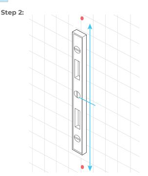
**2.** Mark the place for drilling the hole for the lower post. Mark using a level, in a vertical line from the lower hole, the placement of the upper post hole. Distance approximately 25.7" (653 mm).
