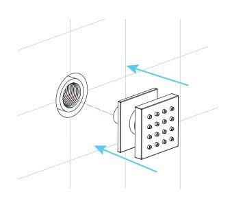
Step 3: Press the escutcheon against the finished wall
