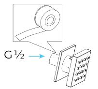
Step 2: Apply teflon tape to threaded tail pipe of the body spray
