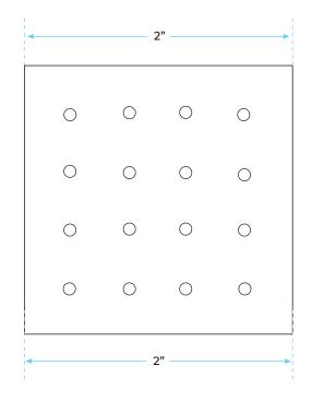
Thread Interface Size: G 1/2 Inch Function: Rainfall Type: Fixed Rotatable Type Installation Type: Wall Mounted Size: 50\* 50 mm(2 inch) Material: Brass Feature: Can rotate 360 degrees Flow Rate: 1.5 GPM / 5.7 LPM (each Bodyspray)
