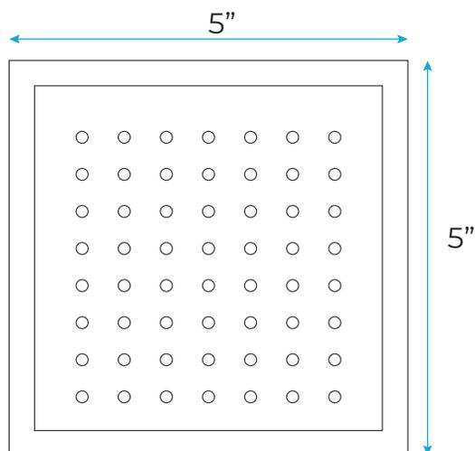
Flow Rate: 1.5 GPM / 5.7 LPM (each Bodyspray)
