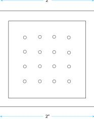
Thread Interface Size: G 1/2 Inch Function: Rainfall Shower Head Feature: Water Saving Shower Heads Type: Fixed Rotatable Type Installation Type: Wall Mounted Size: 50\* 50 mm (2 inch) Material: Brass Feature: Can rotate 360 degrees Flow Rate: 1.5 GPM / 5.7 LPM (each Bodyspray)
